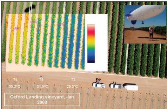
Image 2: Canopy temperature based thermal images in grape vineyards indicating well irrigated and drought affected areas
